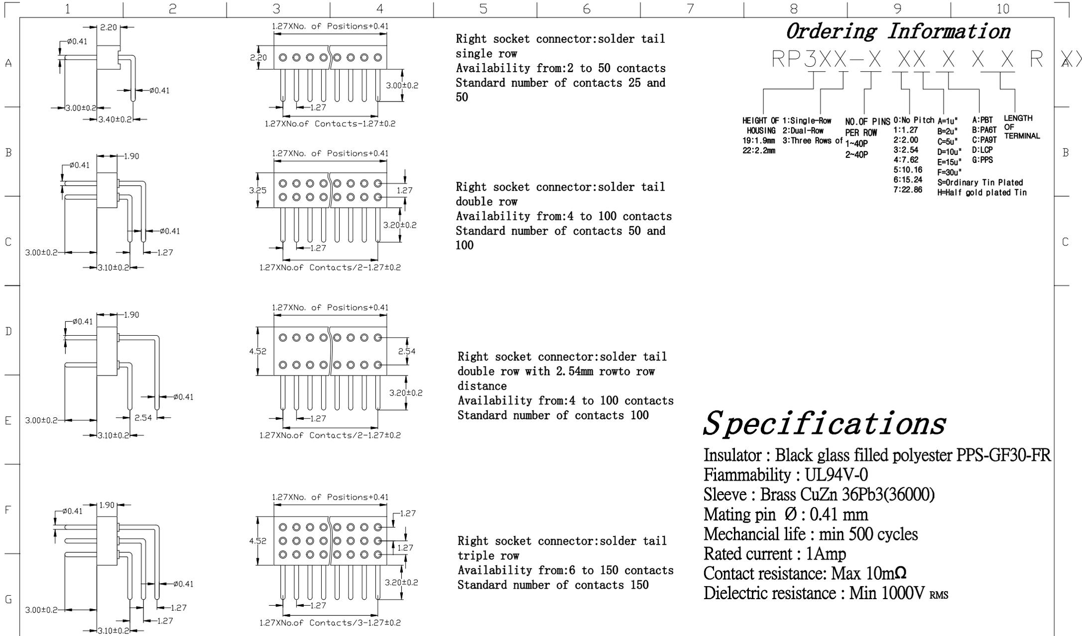
Right socket connector:solder tail
